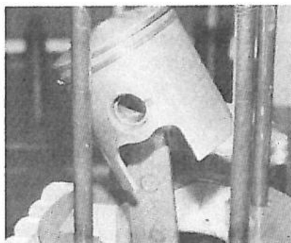
Rotax claim 15 hours racing life for this connecting rod. Maybe polishing could further increase this.
