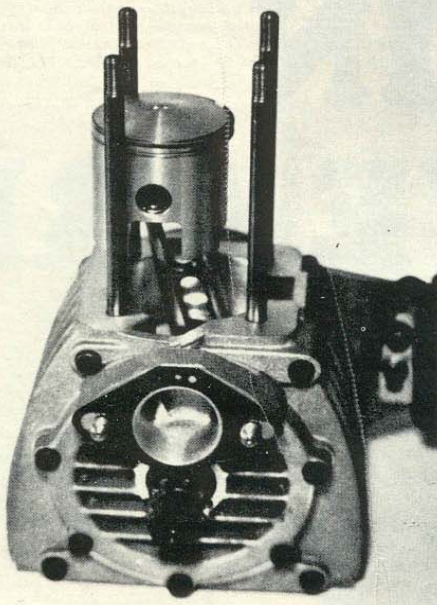
Note the slotted conrod and the larger inlet tract. (Photo by Courtesy of Kart & Superkart).
