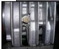
Crankcase has cut away sections between the bottom of the fins . The coil is mounted to the outside .
